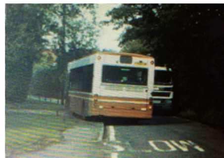
Acorn Street: bus has to mount footpath so HGV can pass.
